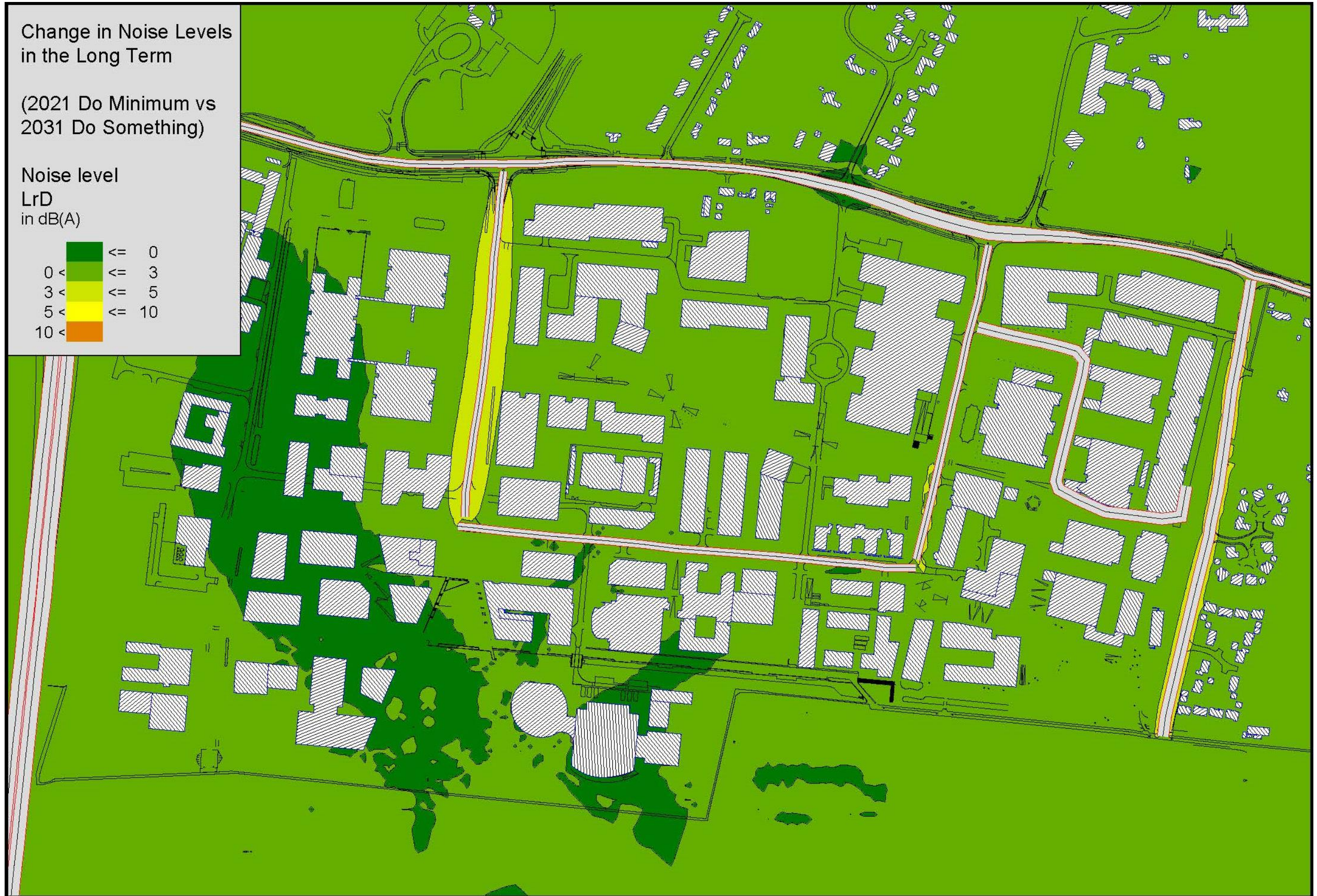
Figure 12.2 Change in noise levels due to road traffic and operational multi-storey car park assessment
