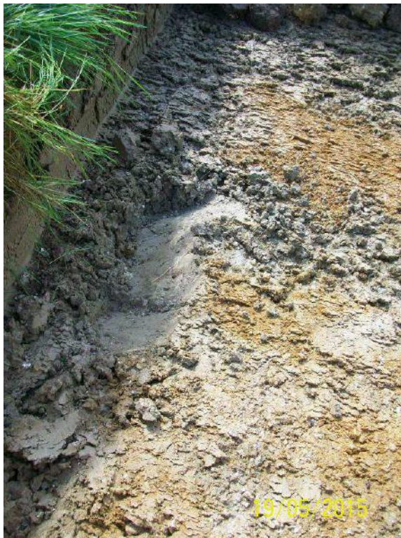
TR4 – Evidence of polished clay surfaces
