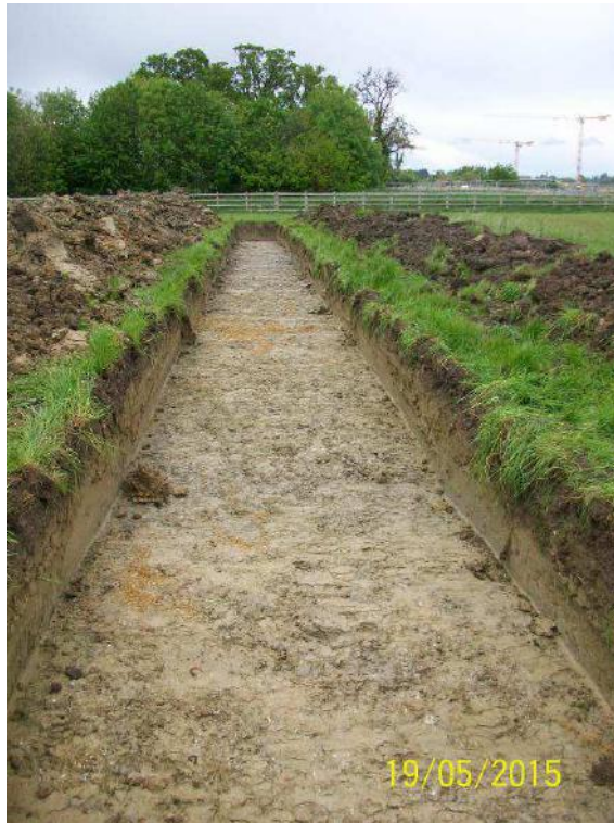
TR5 – Slightly polished clay surfaces observed in this area indicative of possible hill creep / solifluction
