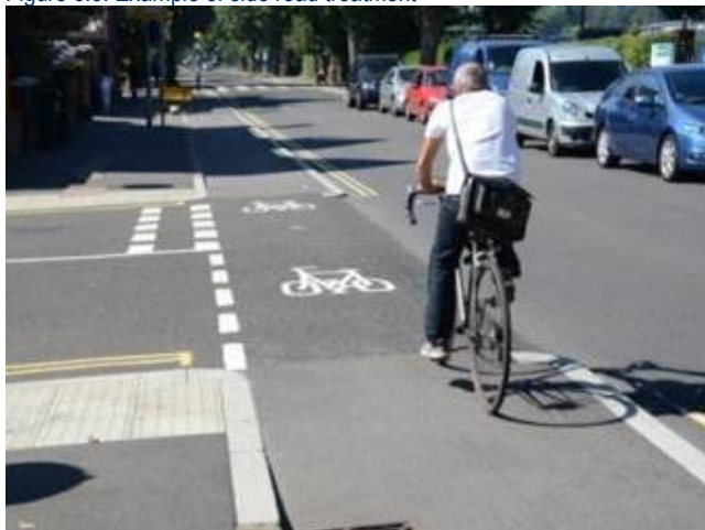
Figure 6.5: Example of side road treatment
